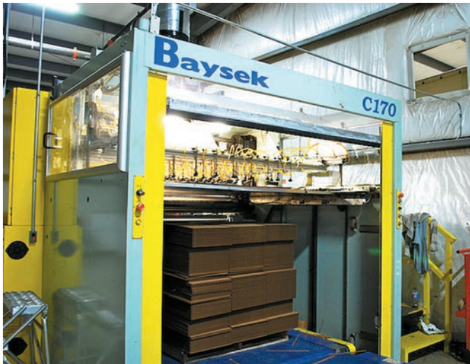
Colepak’s new C-170 flatbed diecutter from Baysek Machines can handle F-flute through doublewall as well as solid and thin board.
