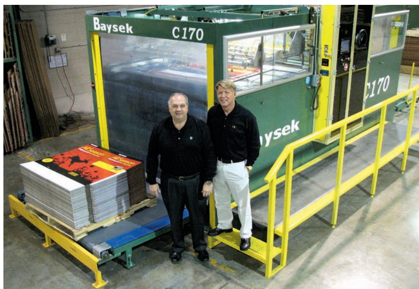
Arrow Box's GM Jess Kramper, left, and owner David Deutschmann have upgraded their product mix, thanks to new equipment like the Baysek C-170 flatbed diecutter.
