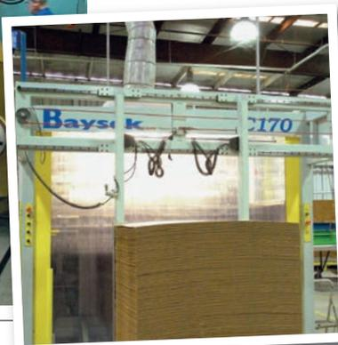
LAST SPRING, MAXPAK INSTALLED A C-170 FLAT DIE, ROTARY ANVIL DIECUTTER FROM BAYSEK MACHINES.
